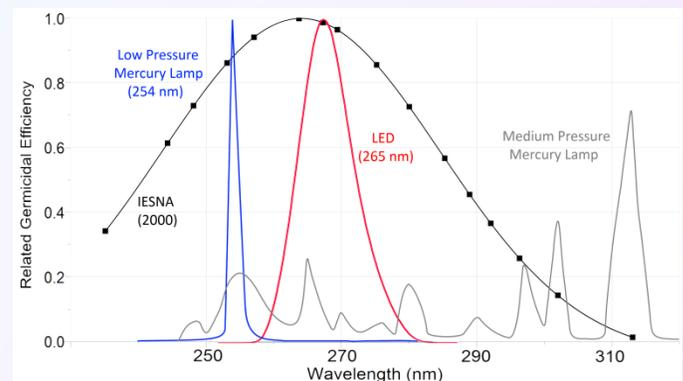
Figure 1: Standardised germicidal response function (black) with superimposed emission spectra of various UV light sources [2].
