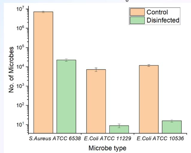
Figure 3: Number of active bacteria in bioaerosol without UV-C treatment (control) and after the treatment at 30 l/min airflow.
